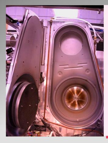
Moderate etch rate High RF bias voltage Low particulate process chamber RF diode etch Ideally suited for applications where large areas of exposed metal and/or silicon are present
